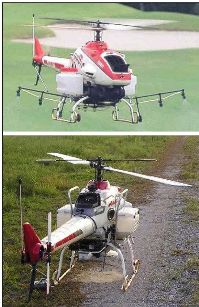
Figure 1. Yamaha RMax unmanned aerial vehicle fitted with ULV spray nozzles (top) and with twin hopper (bottom) for application of granular larvicide to control mosquitoes.
